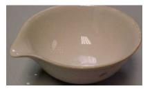
liquids are heated over a flame so that they evaporate, leaving a solid residue
