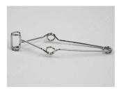
clamp used to hold hot test-tube
