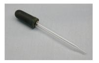
for drawing in a liquid and expelling it in drops
