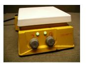
used to heat and stir substances
