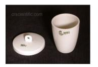
used to hold small amounts of chemicals during heating at high temperatures
